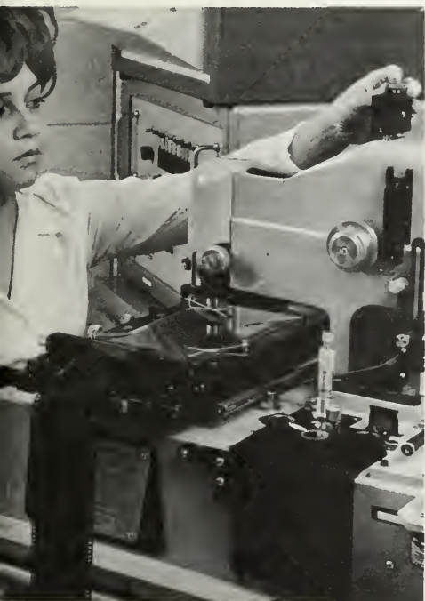
USDA technician operates machine that measures film emulsion density differences in aerial color infrared photos, a technique that may speed collection of surface data from aircraft or satellites.
